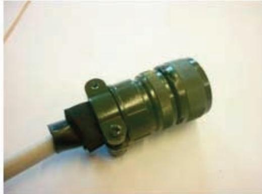
*WICKELN SIE DAS KABEL MIT EINEM MANTEL EIN, UM ES ZU VERDICKEN UND EINES OPTIMALE ANZIEHEN ZU ERHALTEN.*
